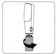
Align the tabs on the bottom of the unit to the top of the cartridge. Screw in the cartridge until you feel it click into place.
