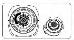
If necessary, remove the cartridge adapter by turning it and cleaning it with your fingers using water and mild soap.
