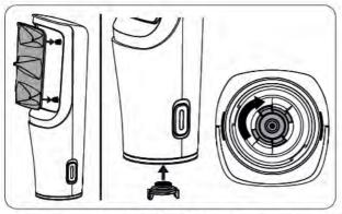
Allow all parts of the IONIQ ONE to dry completely before reassembling. Replace the cartridge adapter and nozzle field. Press each nozzle down individually so that the nozzle array is fully engaged and sits completely flush on the sprayer.
