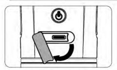
Slide the cover to the side. Plug the USB cable into the switchedoff appliance and connect it to the power source.
