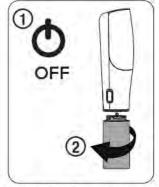
Switch off the appliance and remove the cleaning cartridge.
