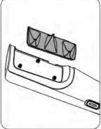
Remove the nozzle field and clean thoroughly under running water with mild soap by pressing/ rubbing.
